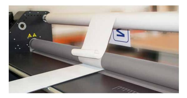
Start mounting by some push of the board to move between the axles and push "start"- key. Move away liner manually during mounting process.
