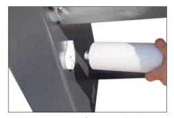
insert this end of the scroller into the left connection
