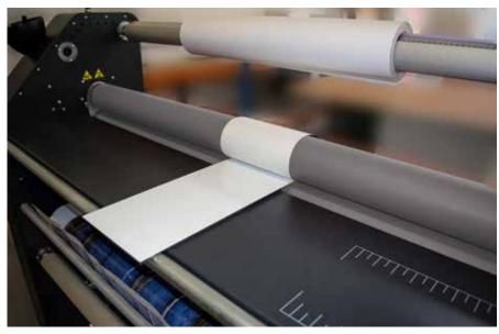
Cut the liner of one half of the self adhesive media and mount this half by using the laminator pushing "start" key.
